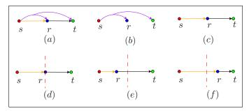
Fig. 2. (a): One receiver case decomposed into two subgraphs from s to t, (b) and (c), respectively. (d): Optimal position of r for  $P_s = P_r$  and  $\alpha = 2$ , which is at the perpendicular bisector (red) of line segment s-t. (e): Left bias for  $P_s < P_r$ . (f): Right bias for  $P_s > P_r$ .
